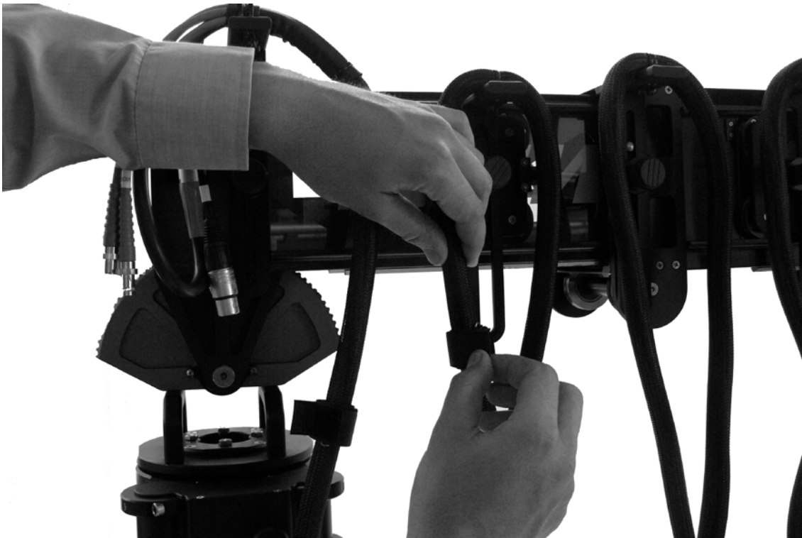
2.12.1.a - Mounting additional cables at wagon
