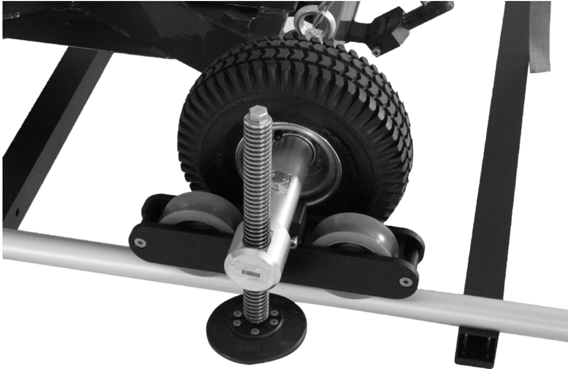
2.2.3.b - Track wheels moving on tracks
