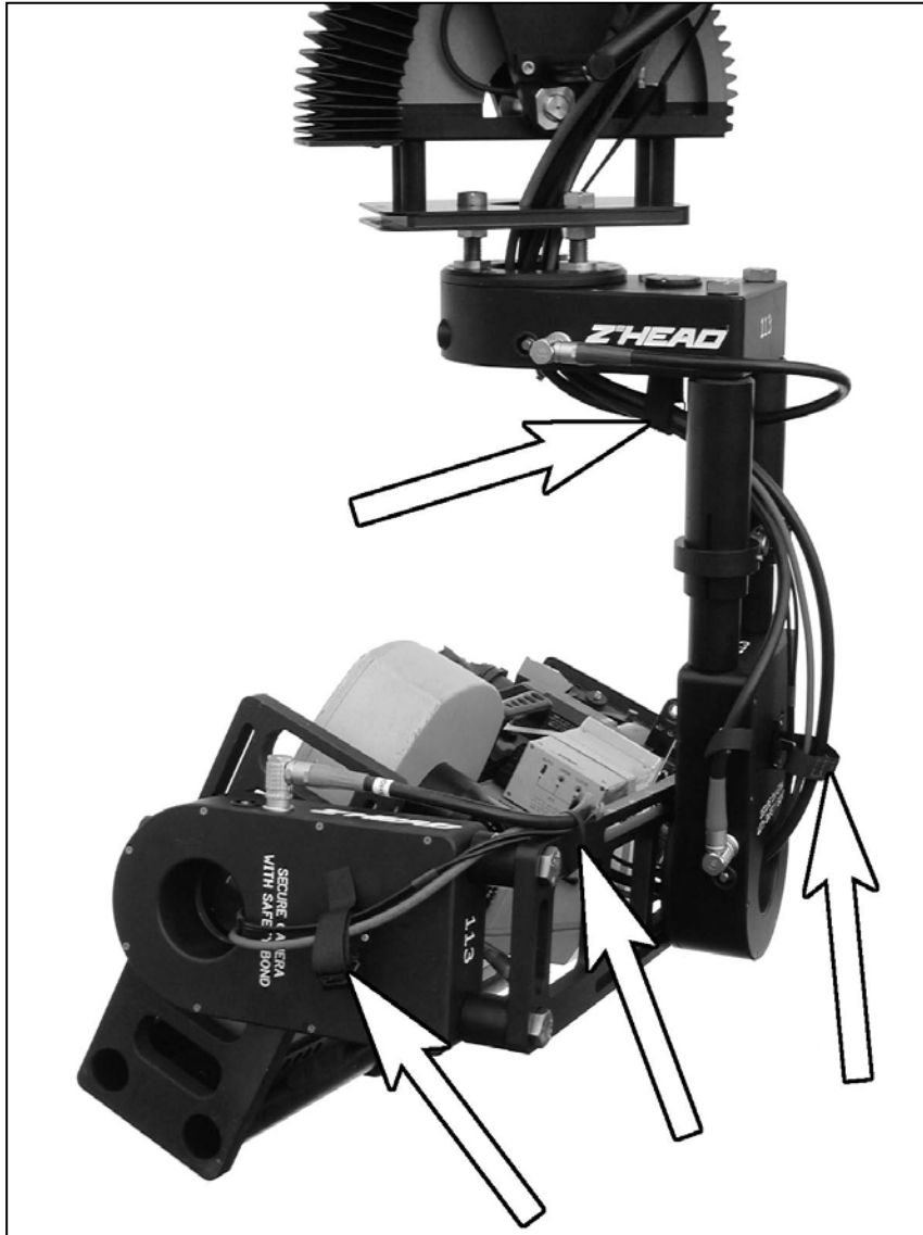
2.8.7.b - Recommended fixing points for cables
