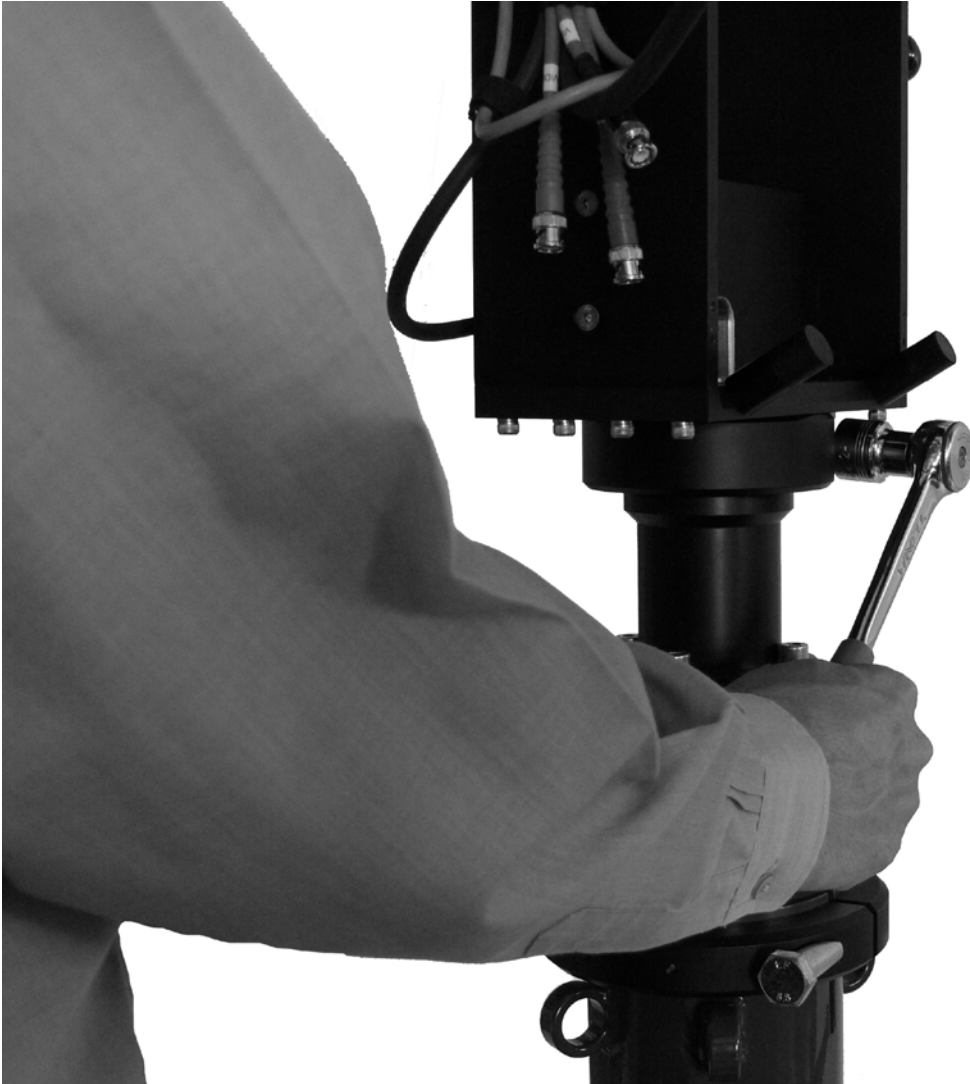
2.3.4.c - Locking the horizontal brake
