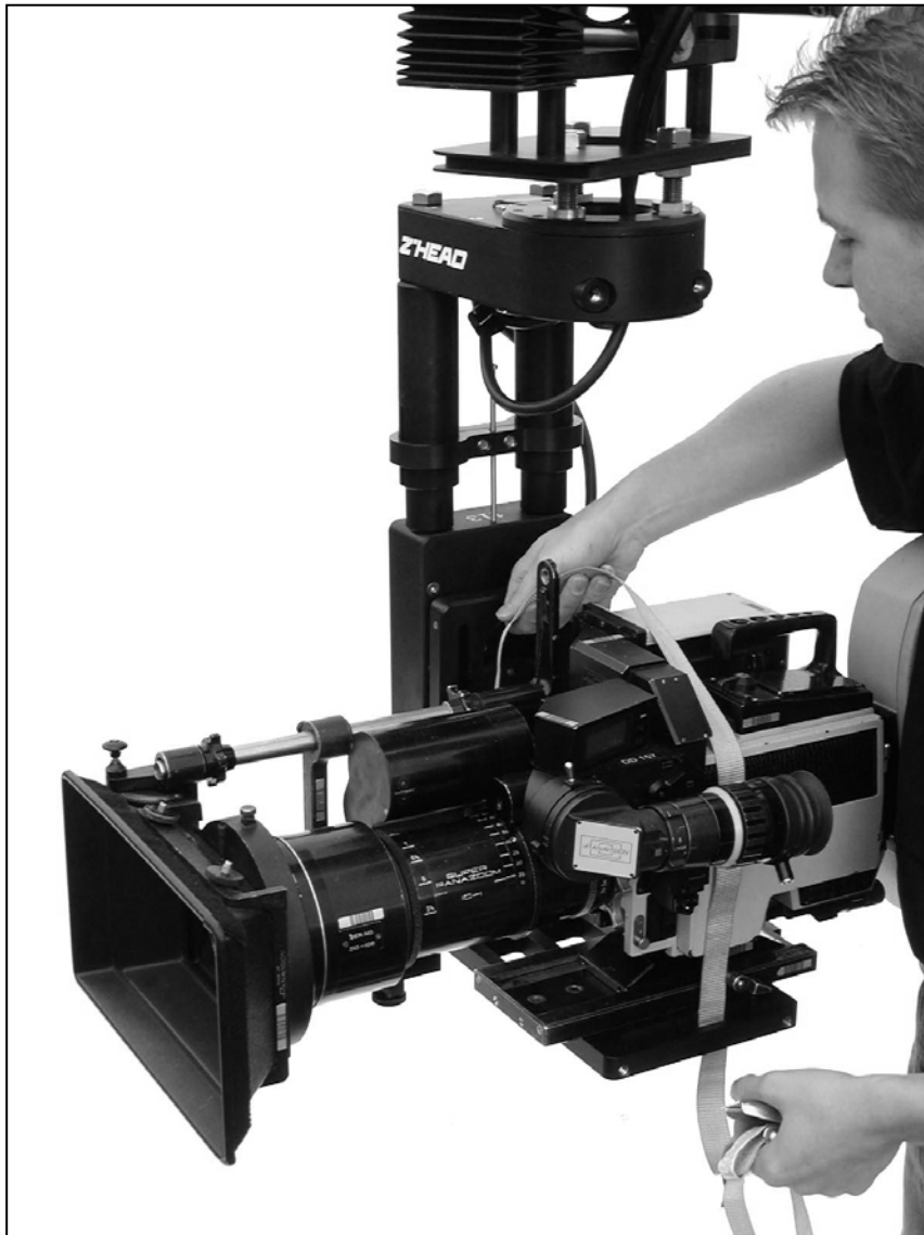
2.8.2.b - Securing the camera with a strap
