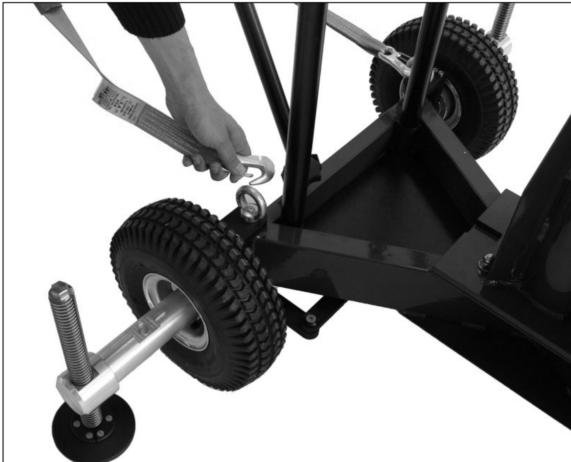
1.1.a - Snap hook at eyebolt on dolly
