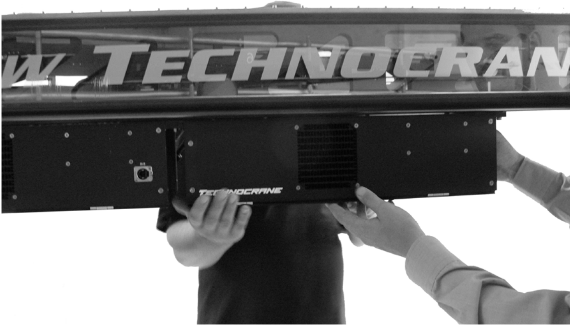
2.9.1.a - Lifting unit into crane
