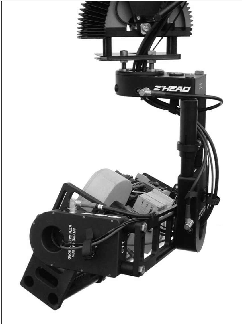
2.8.7.a - Cables at pan, tilt and roll
