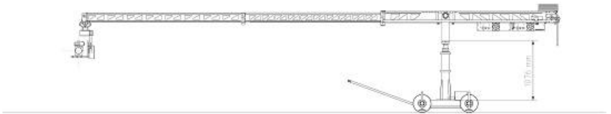
2.3.4.a - Drawings of the crane extended, one with column in, one with it out
