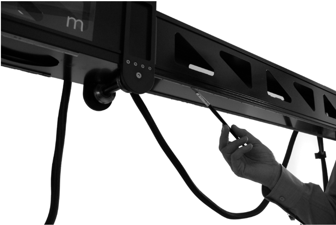
2.5.1.e – Greasing the tracks with a brush
