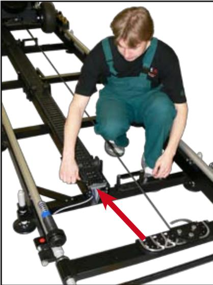
2.2.6.d. - Attaching the cable carrier to a sleeper
