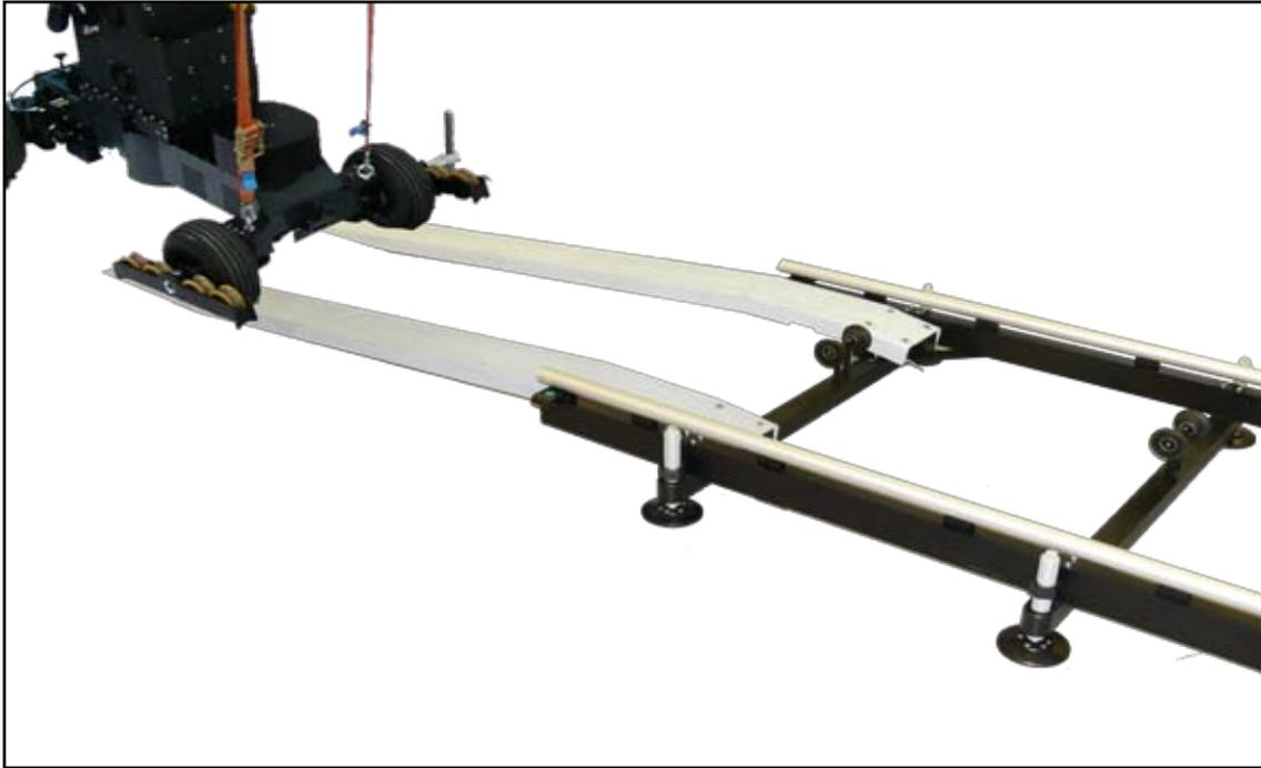
*2.2.4.b – Base moving onto the ramps*
