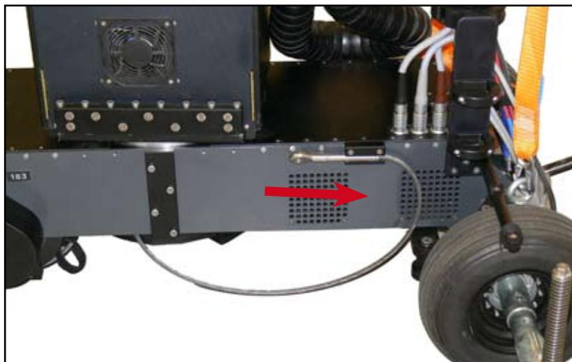
12. Restore the wire in the nest after shooting in order to avoid any damage to the wire.
