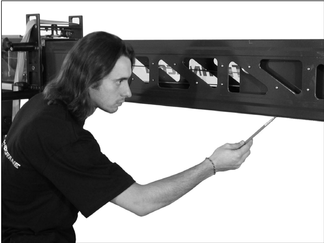
2.5.1.e – Greasing the tracks with a brush
