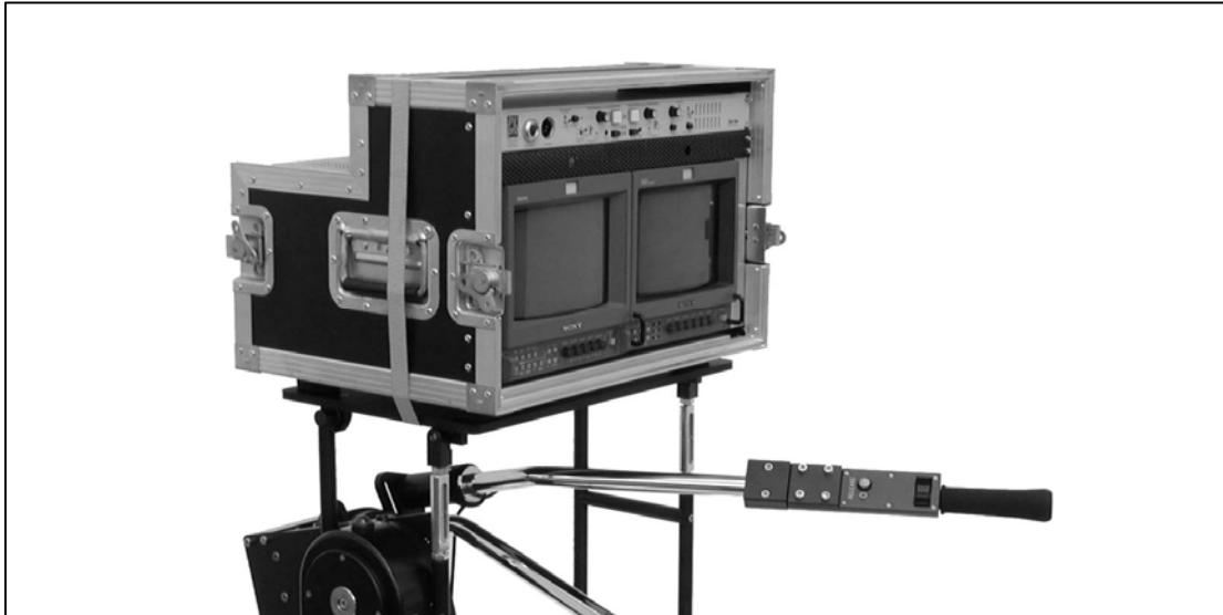
2.16.2.e - Two monitors on pan bars with straps
