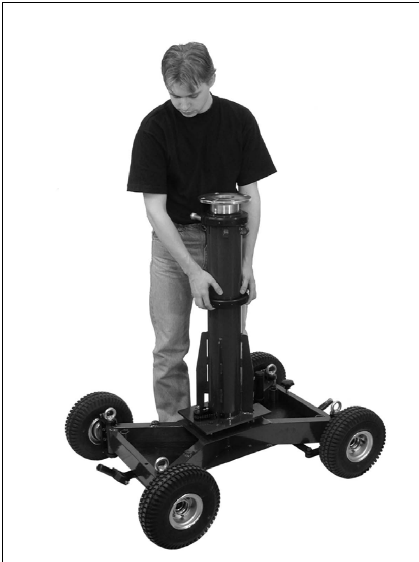
2.3.1.a - Placing column onto the dolly
