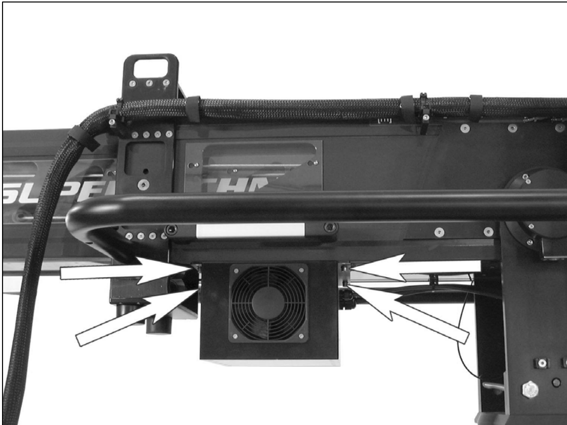
2.11.2. Screws on speed box
