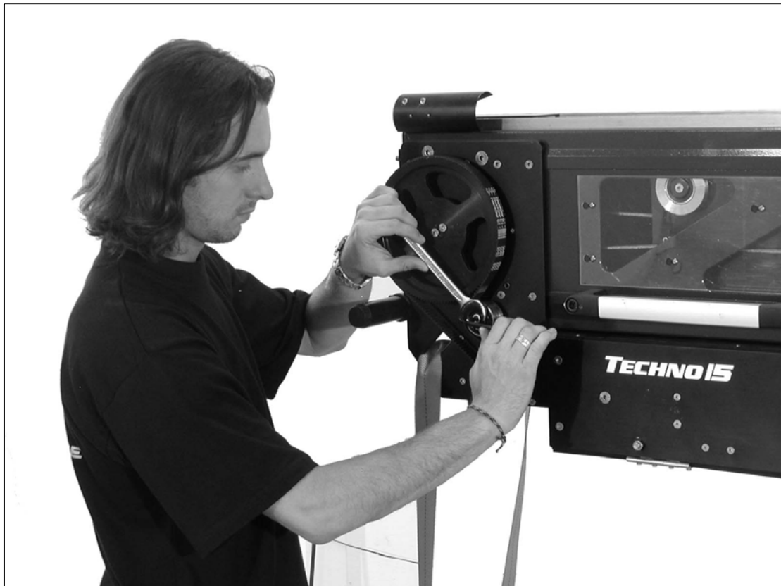
2.6.2 - Adjusting the eccentric pulley
