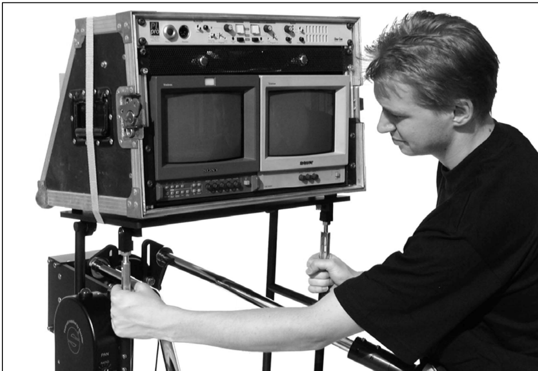
2.16.2.f - Setting the monitor angle with studs
