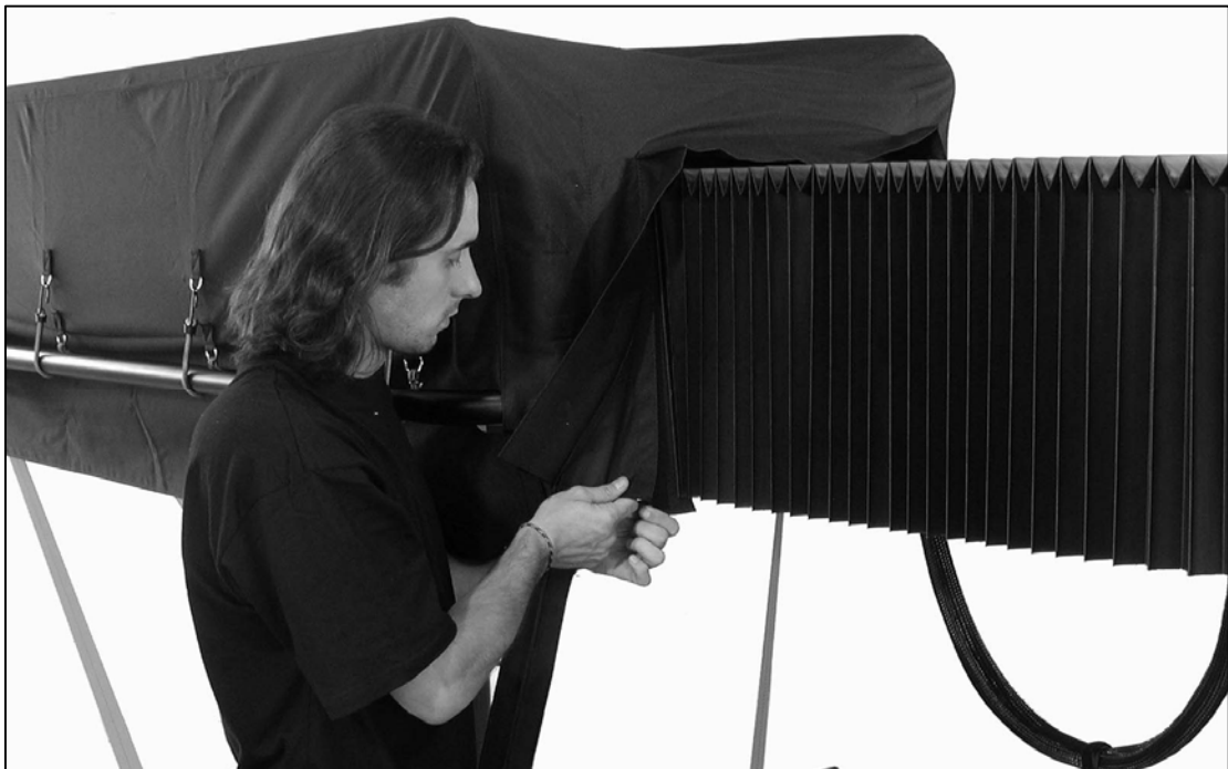
2.13.3.g -Fixing front part of cover for first beam
