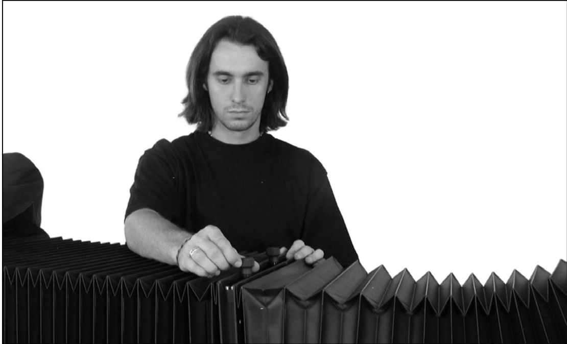
2.13.3.f - Mounting bellows frame on second beam
