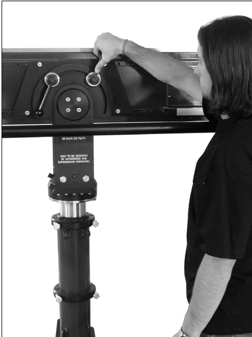
2.3.6.a - Locking tilt brakes
