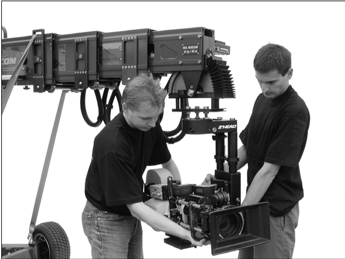
2.9.2.a - Mounting camera at base plate
