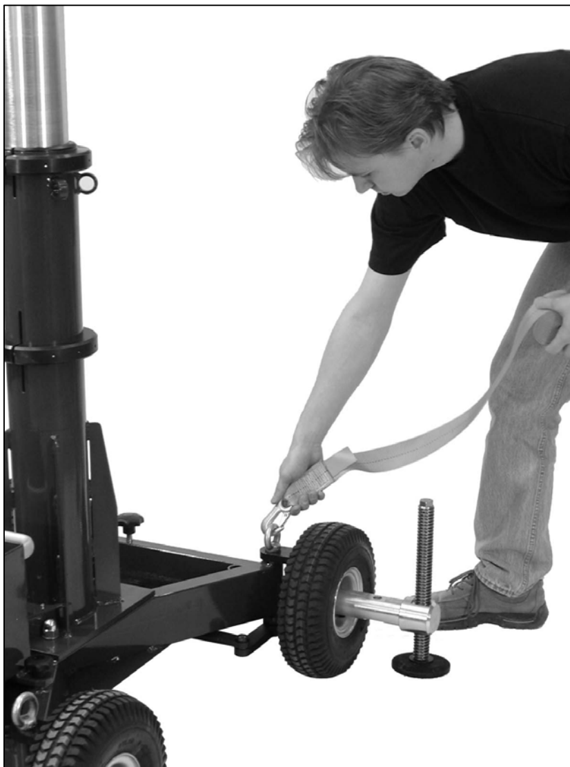
1.1.a - Snap hook at eyebolt on dolly
