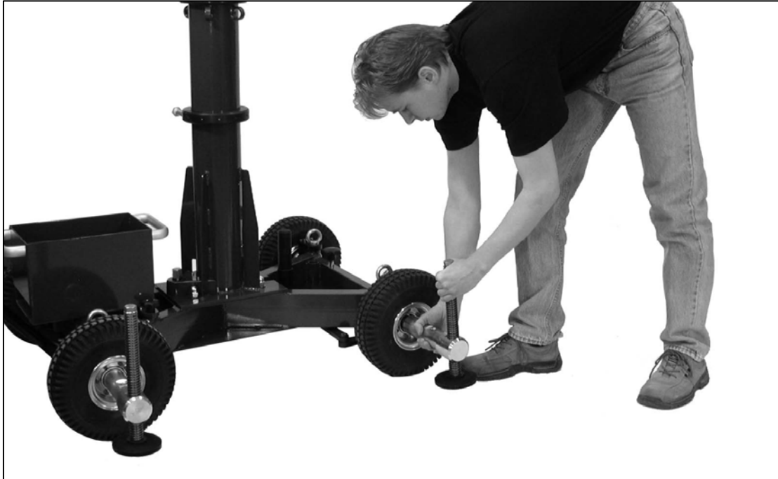
2.1.2.a - Jack moving into wheel
