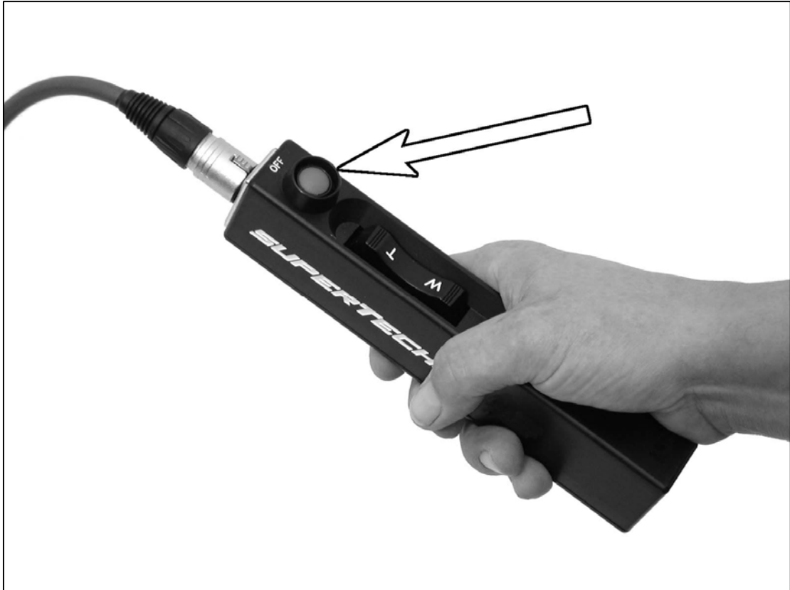
2.12.1.d - Red button at hand control
