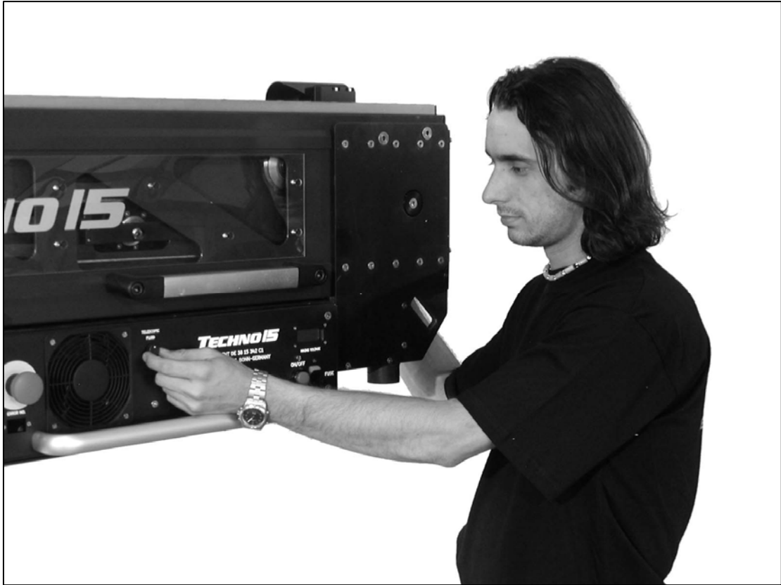
2.12.1.c - Turning fluid potentiometer at electronic unit
