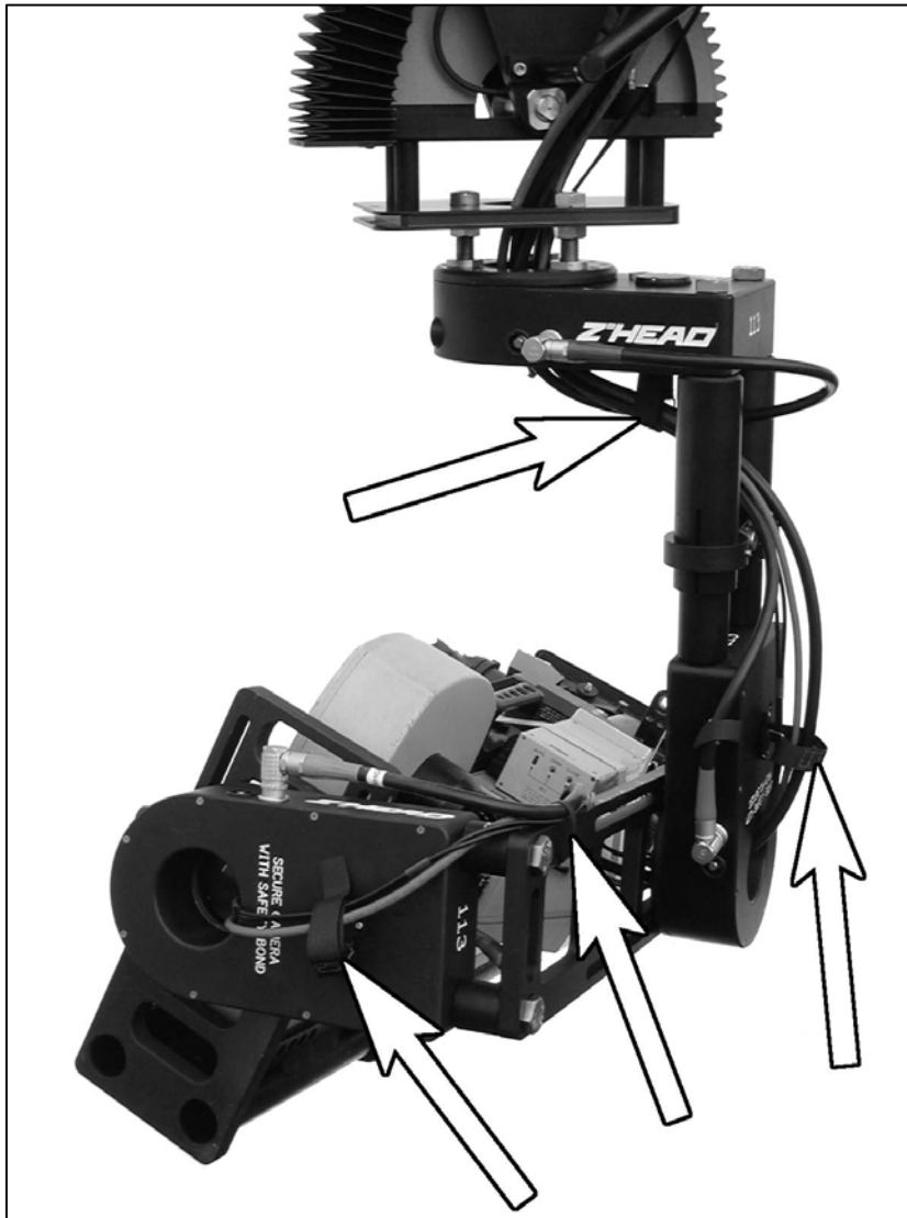
2.9.7.b - Recommended fixing points for cables
