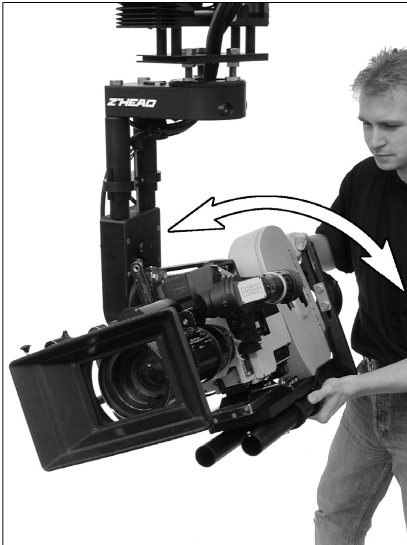
2.9.6.a - Camera moving on roll left and right
