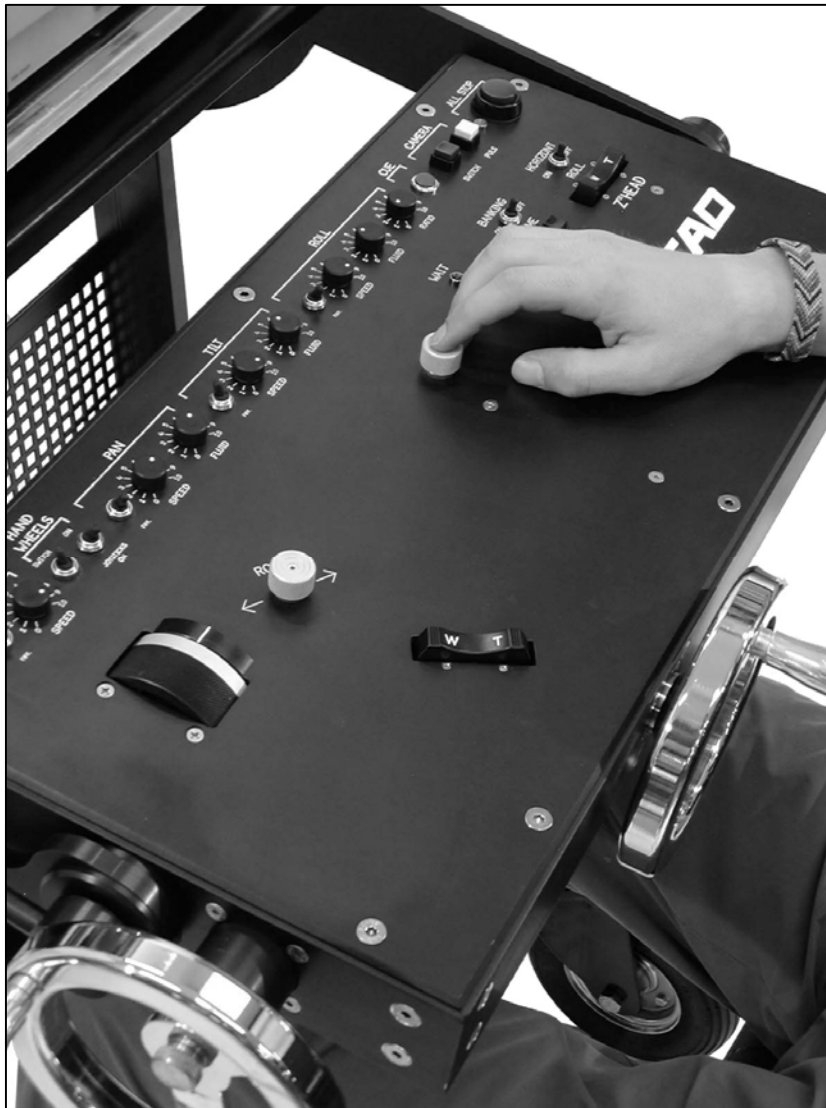
2.14.5.a – Pan-tilt joystick
