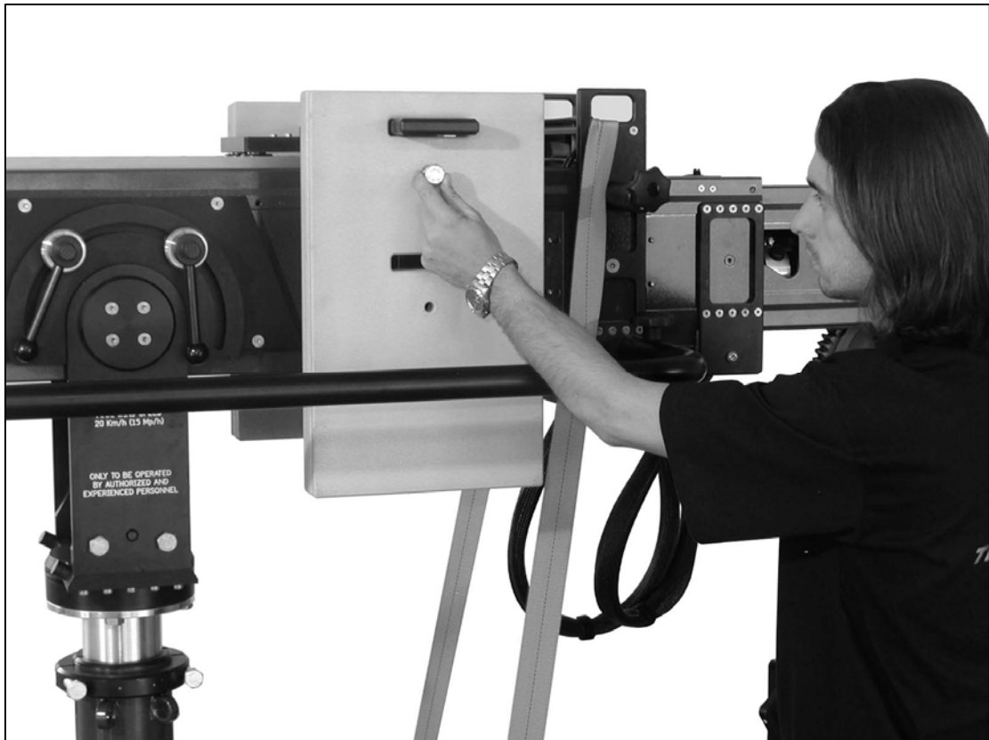
1.3. - Putting M16 hexagon head at counterweights
