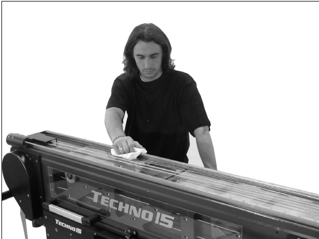
2.5.1.g - Cleaning the counterweight tracks
