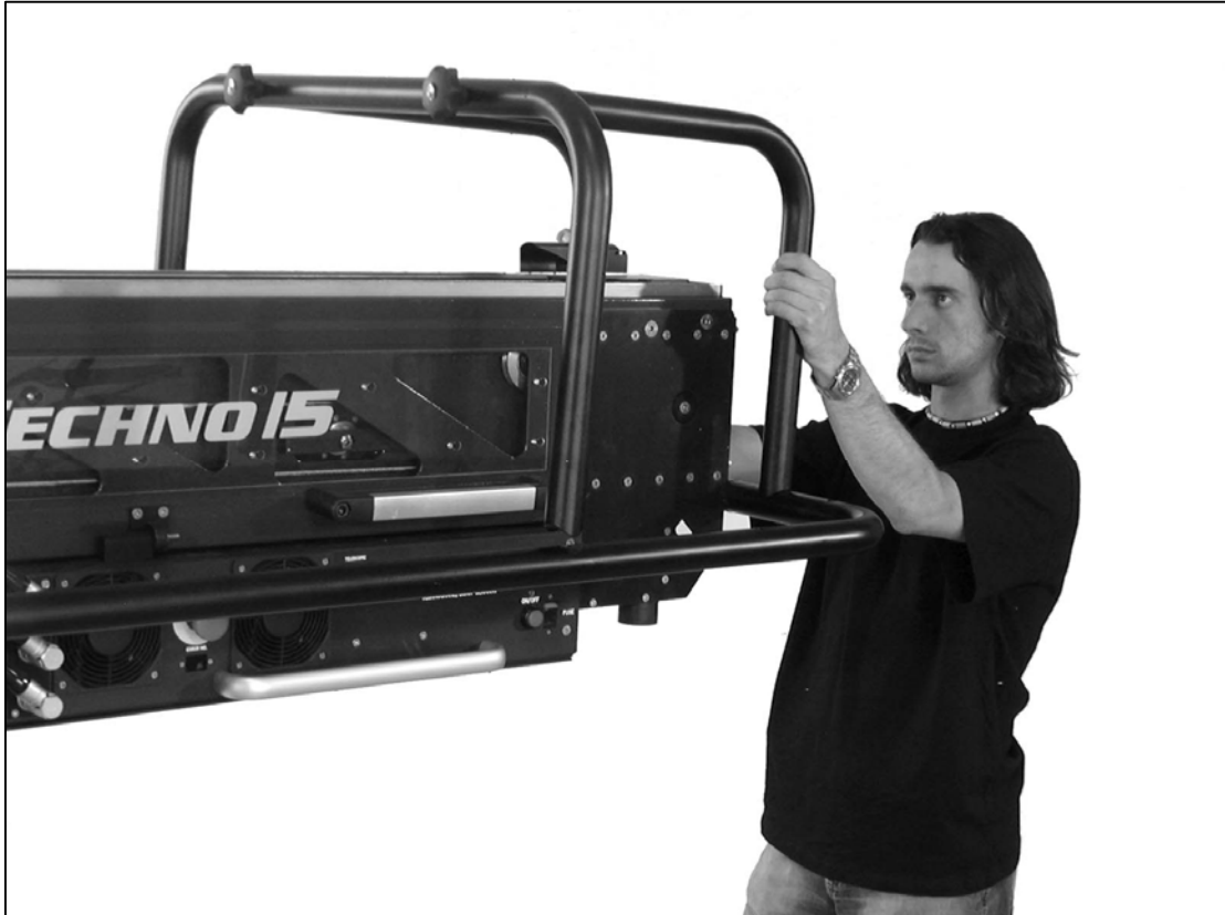
2.13.1.a - Taking the back tubes off
