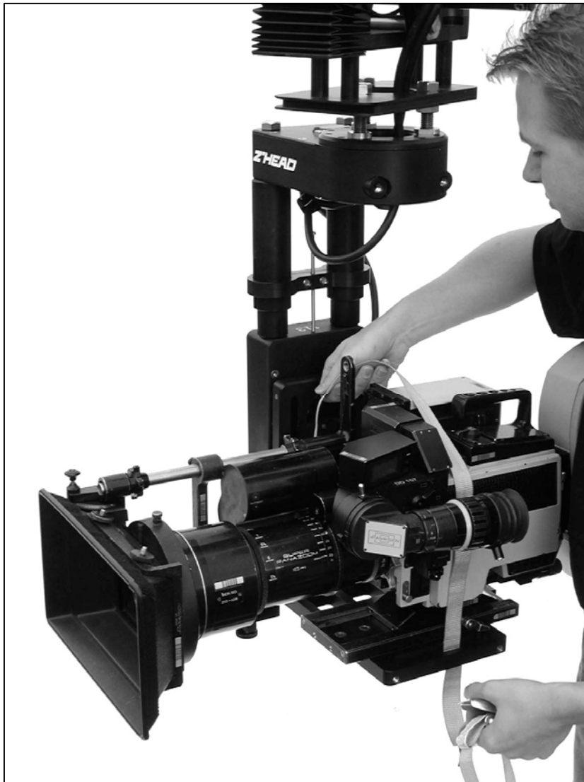
2.9.2.b - Securing the camera with a strap
