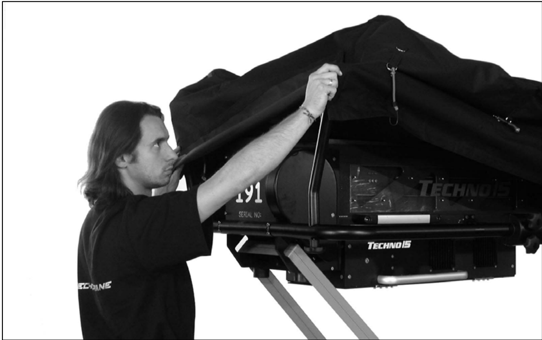
2.13.1.d - Putting cover over the first beam
