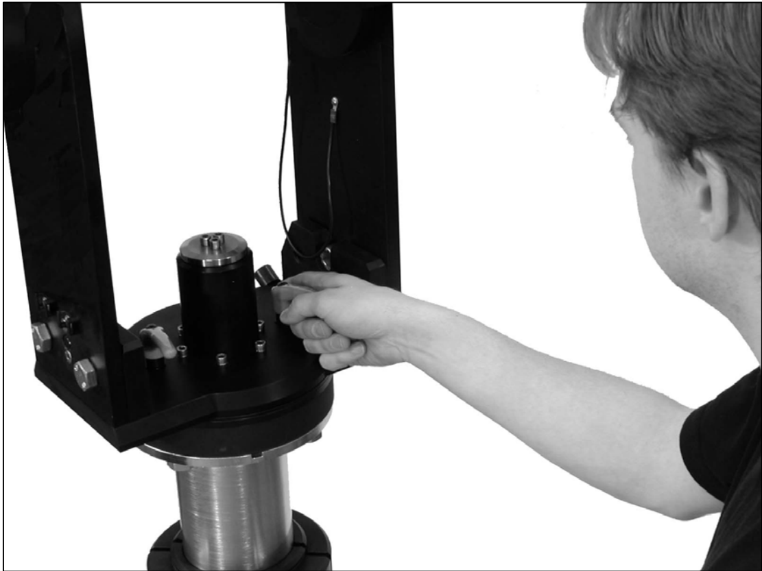
2.3.4.c - Locking the horizontal brake
