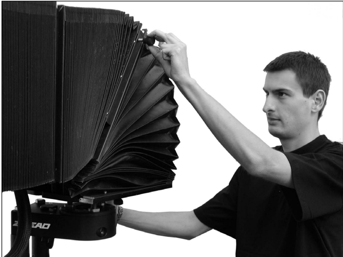
2.13.3.e - Attaching bellows frame at fourth beam
