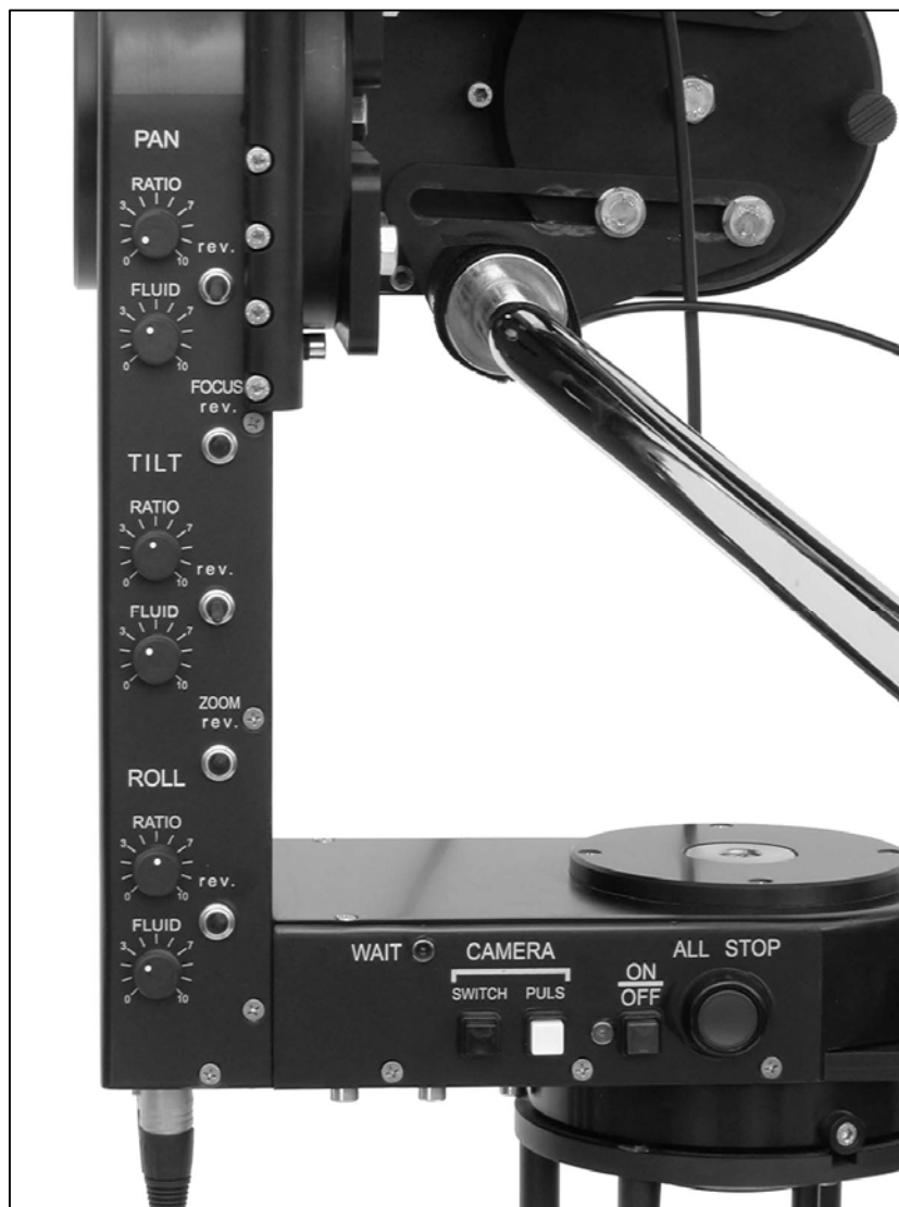
2.16.4.b - Front view of pan bars with potentiometers
