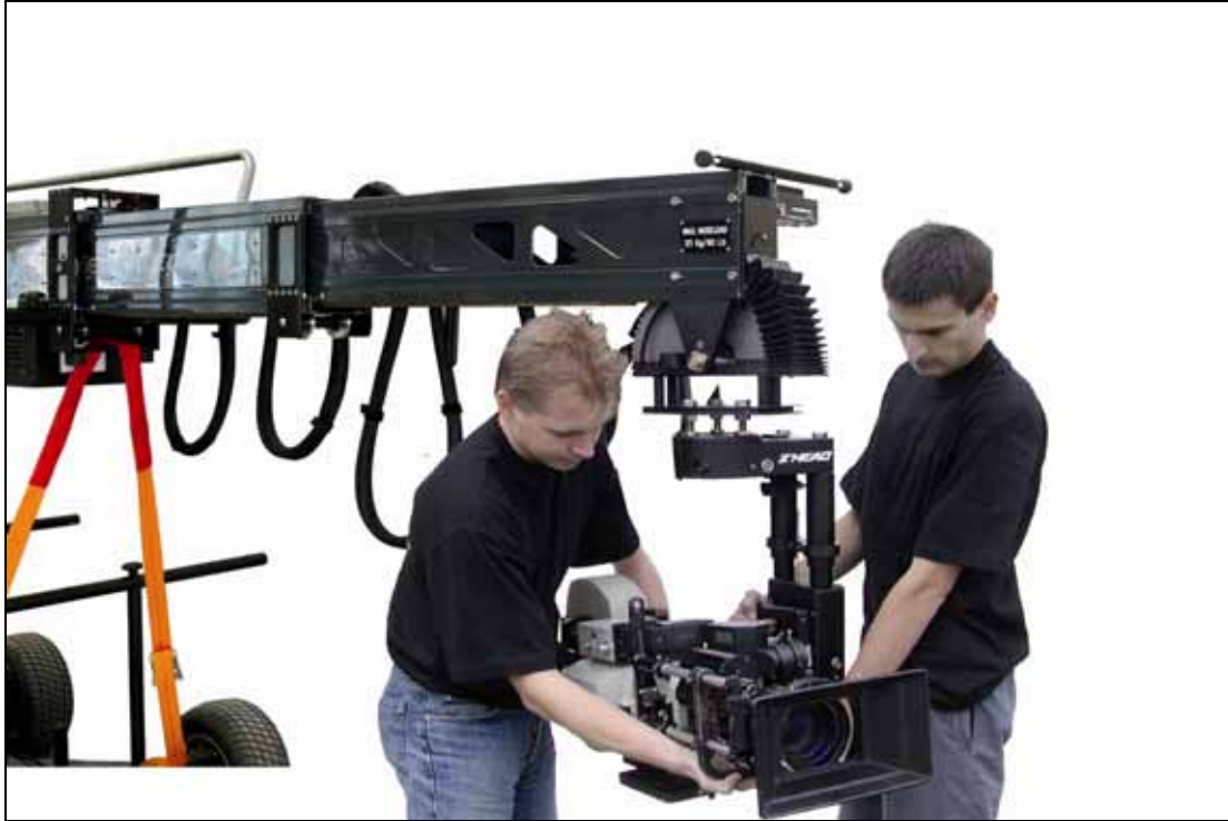
2.9.2.a - Mounting camera at base plate
