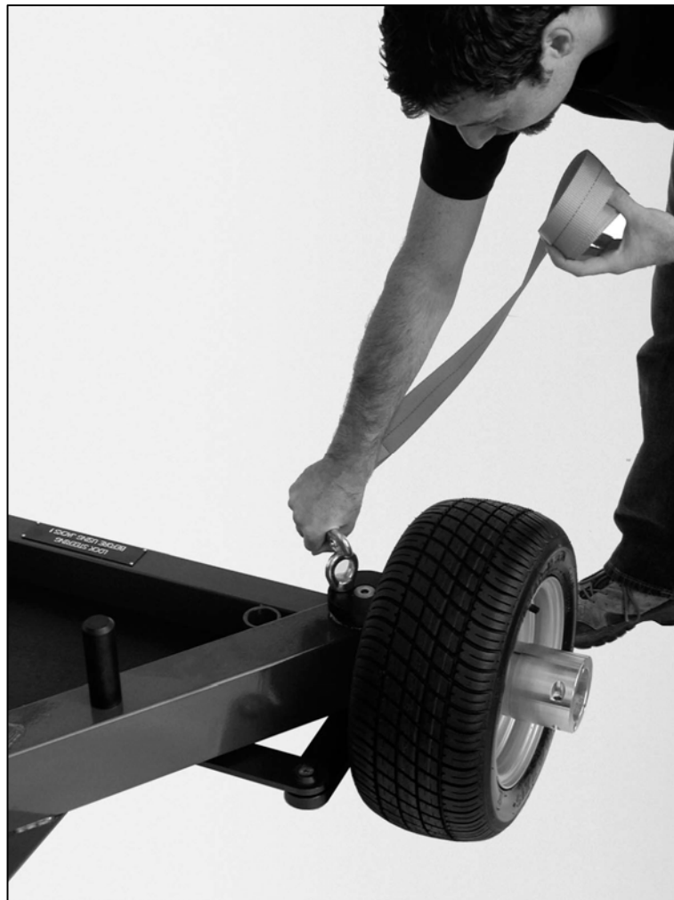
1.1.a - Snap hook at eyebolt on dolly
