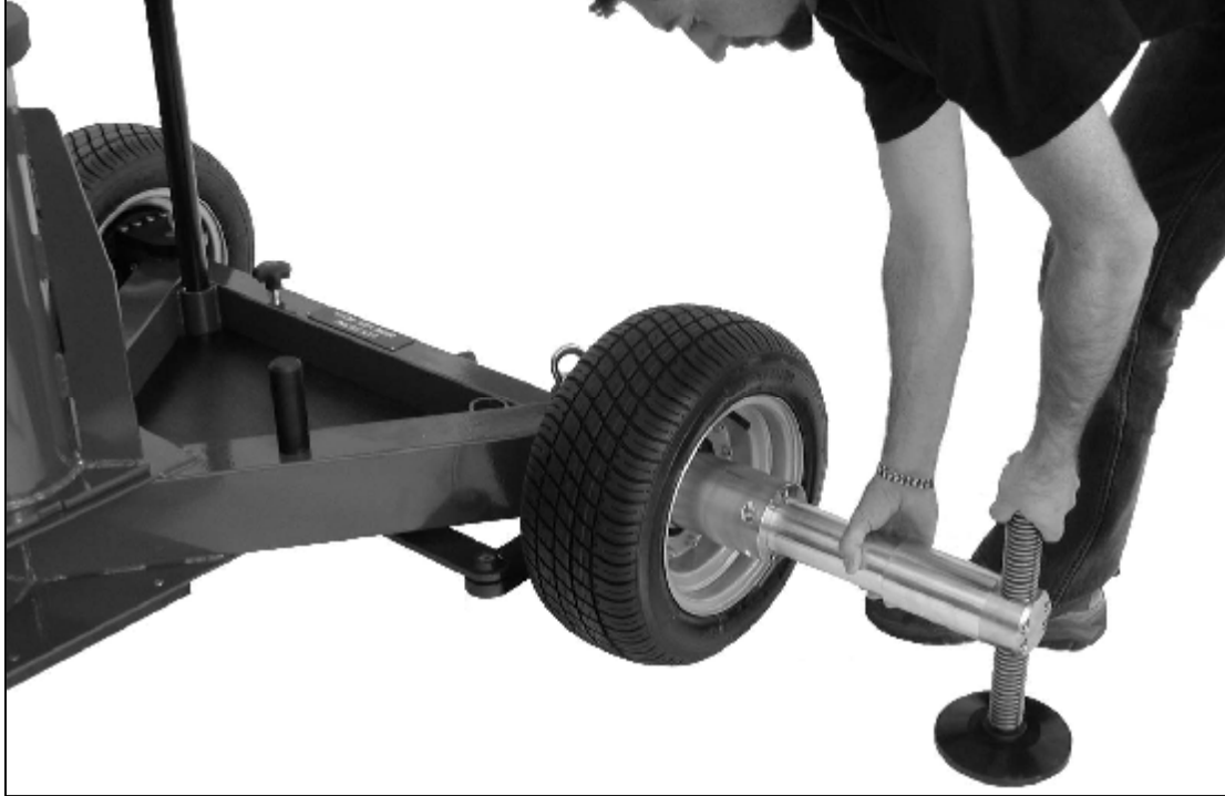
2.1.2.a - Jack moving into wheel
