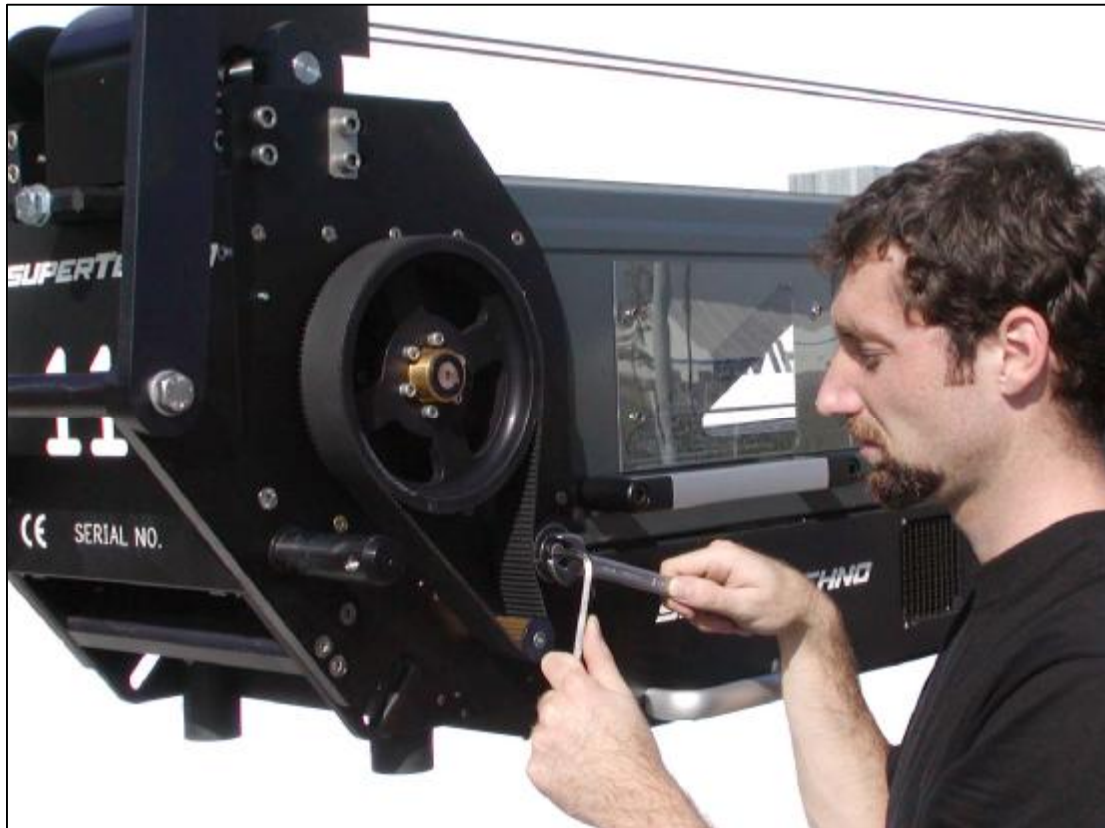
2.6.2 - Adjusting the eccentric pulley
