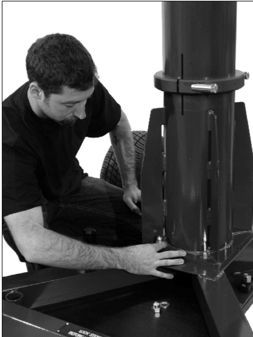
2.3.1.b - Nuts being fitted
