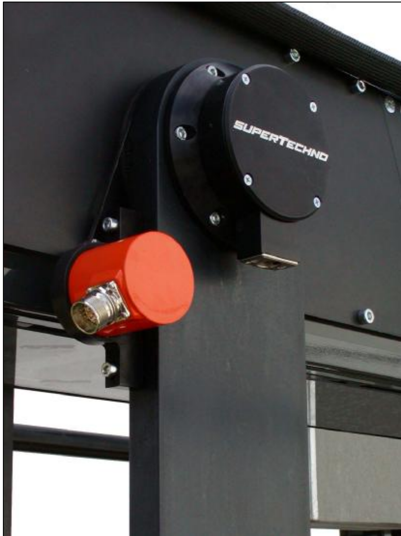
2.3.8.b - Encoder at crane tilt
