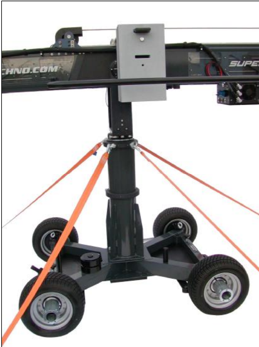
2.3.3 - Four eye screws with snap hooks
