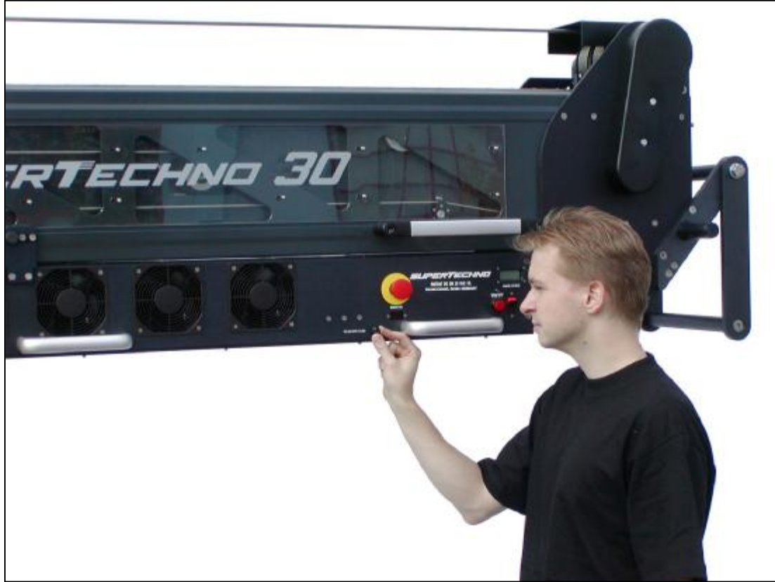
2.12.1.c - Turning fluid potentiometer at electronic unit
