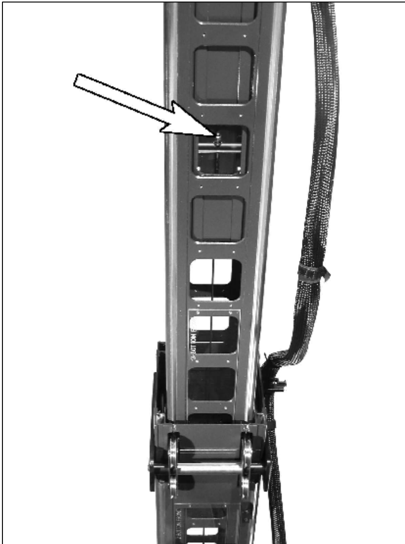
2.6.1.f - Anchorage pull in cable (4 th beam section)
