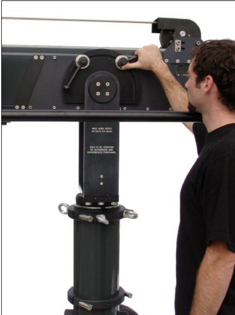
2.3.6.a - Locking tilt brakes
