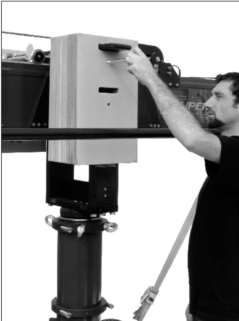
1.3. - Putting M16 hexagon head at counterweights
