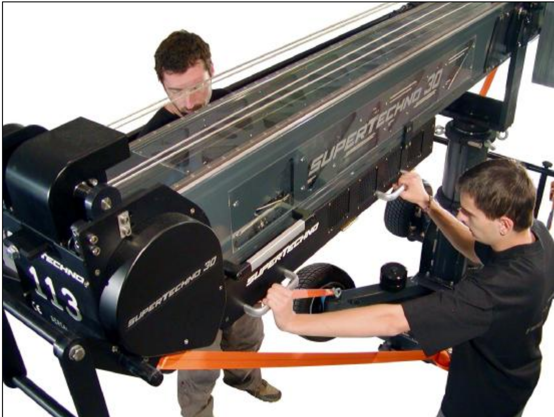
2.10.1.a - Lifting unit into crane
