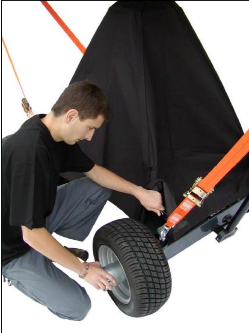
2.15.2.b - Fixing to eyebolts and closing tent
