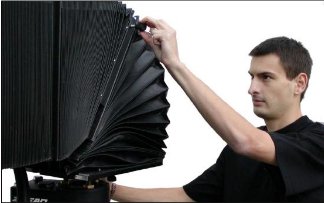
2.15.3.e - Attaching bellows frame at fourth beam
