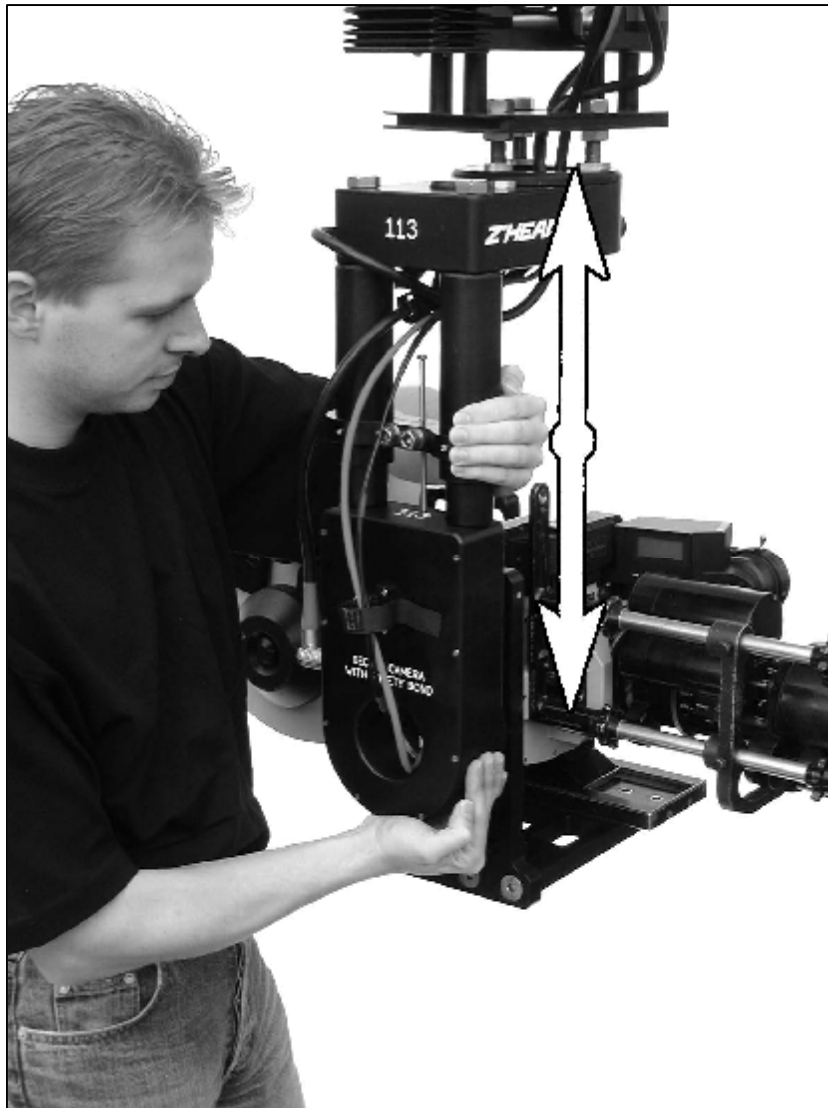
2.9.4. – Moving raiser up and down
