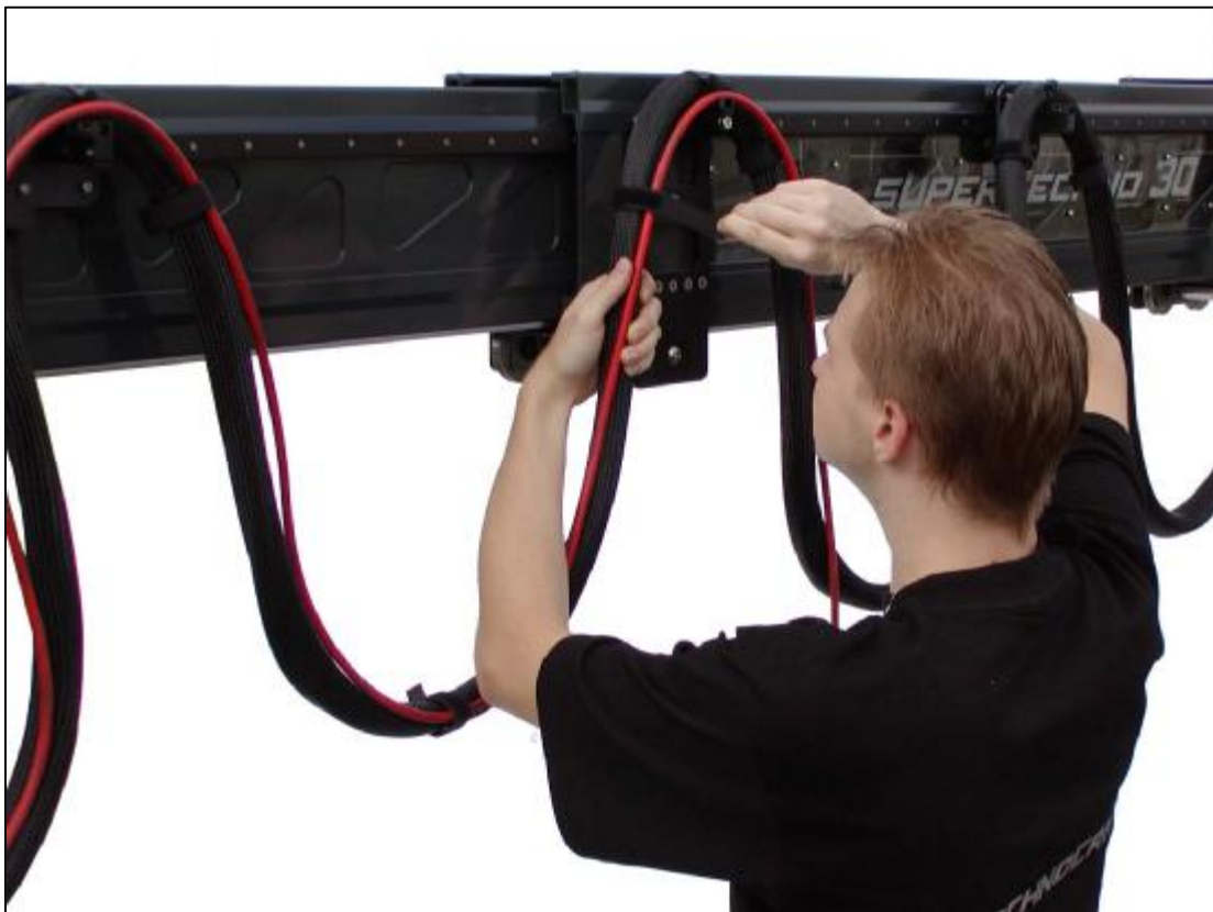
2.14.1.a - Mounting additional cables at wagon
