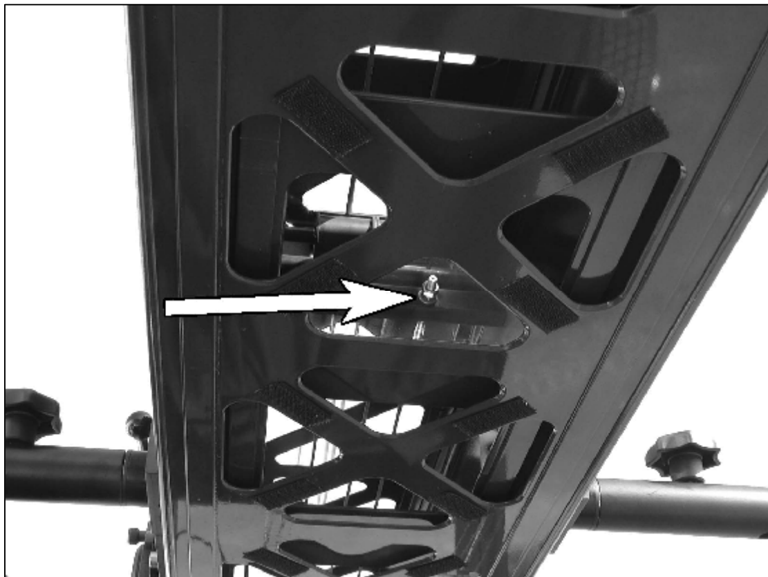
2.6.1.d - Anchorage pull in cable (2 nd beam section)
