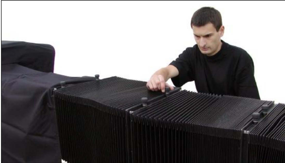
2.15.3.g - Mounting bellows frame on second beam
