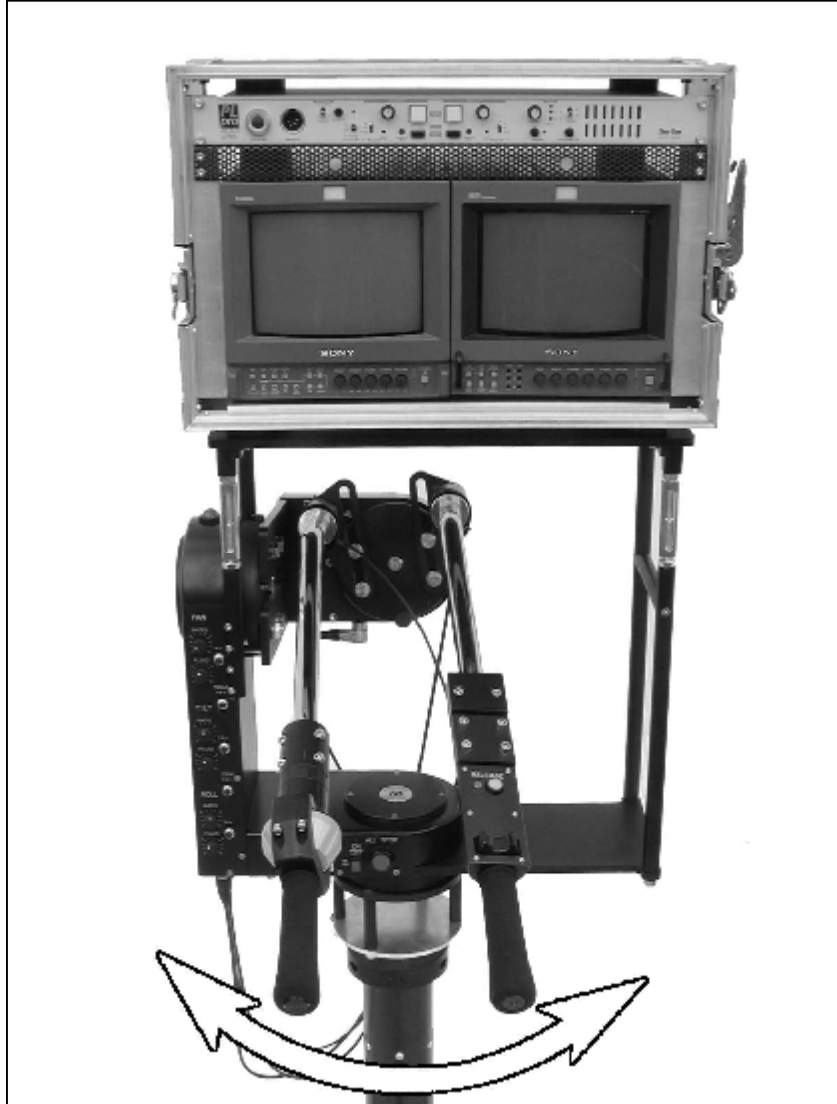
2.18.2.h - Arms together (min. separation)
