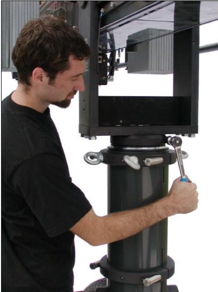
2.3.4.c - Locking the horizontal brake
