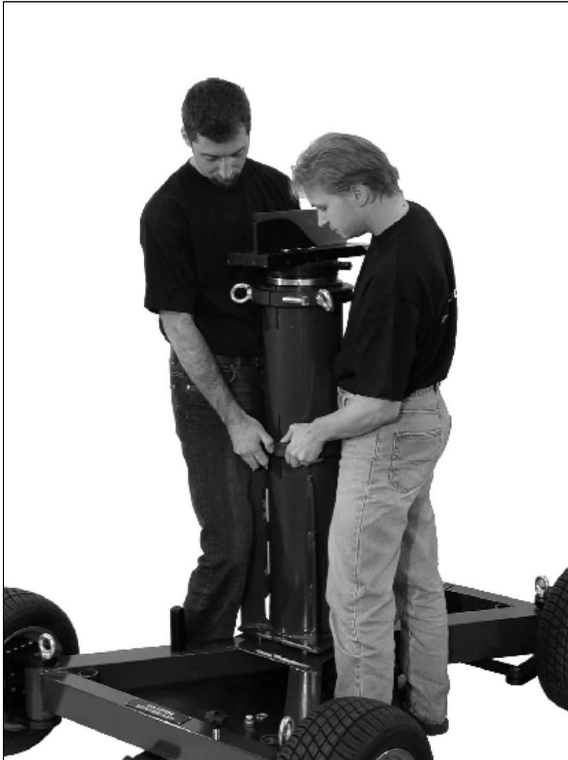
2.3.1.a - Placing column onto the dolly
