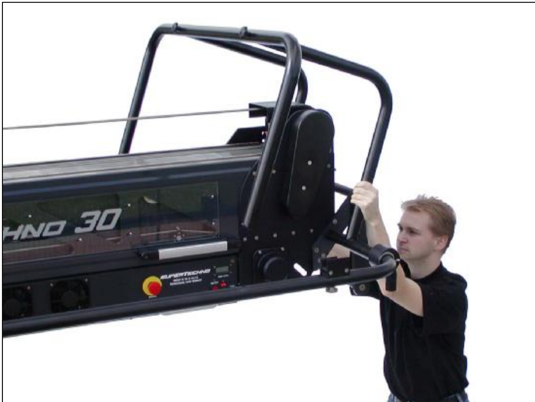
2.15.1.a - Taking the back tubes off
