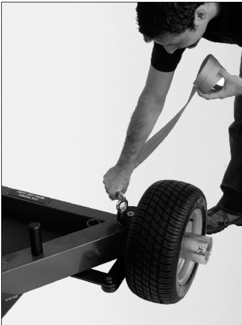
1.1.a - Snap hook at eyebolt on dolly
