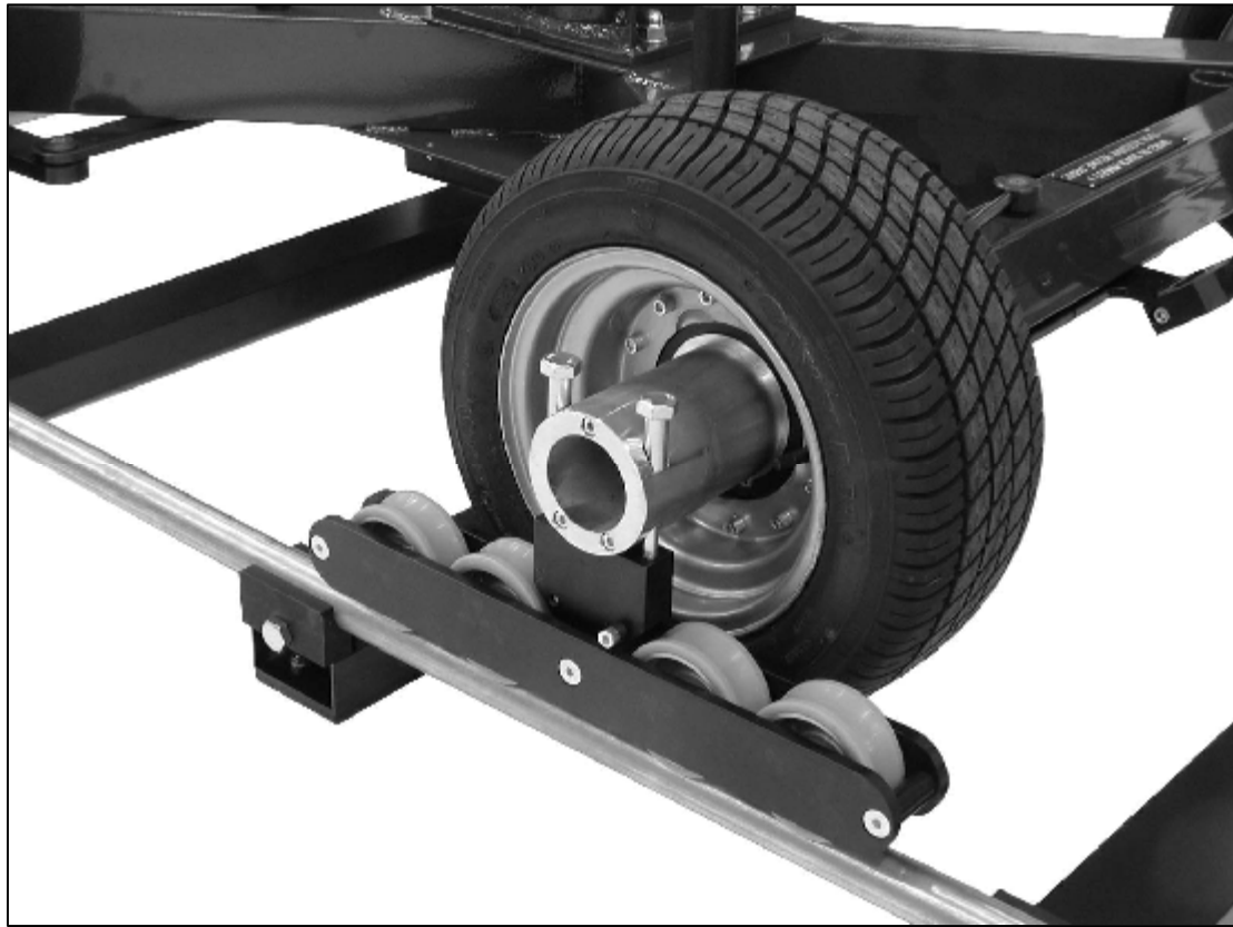
2.2.3.b - Track wheels moving on tracks
