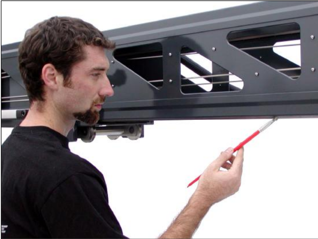
2.5.1.e – Greasing the tracks with a brush
