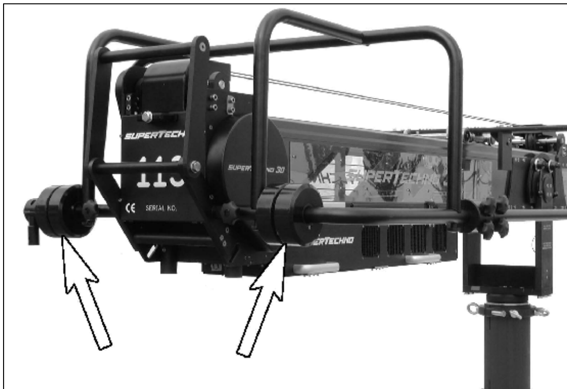
2.7.1.d - Four donuts at the back of the crane
