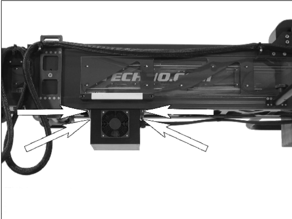
2.11.2. - Screws on speed box
