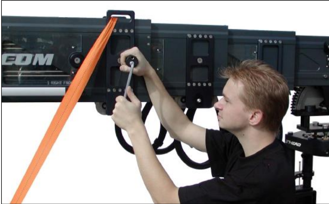
2.15.1.b - Taking off donut holder at first beam
