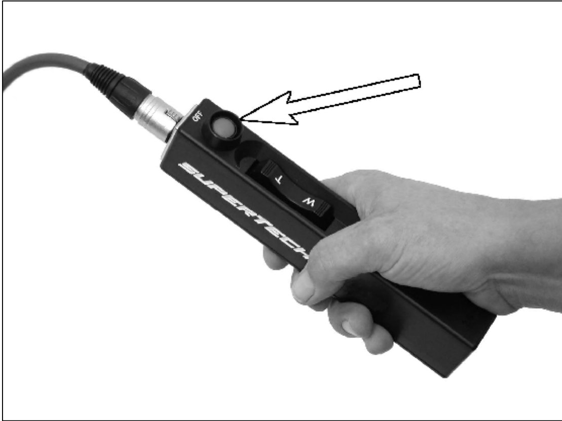
2.12.1.d - Red button at hand control
