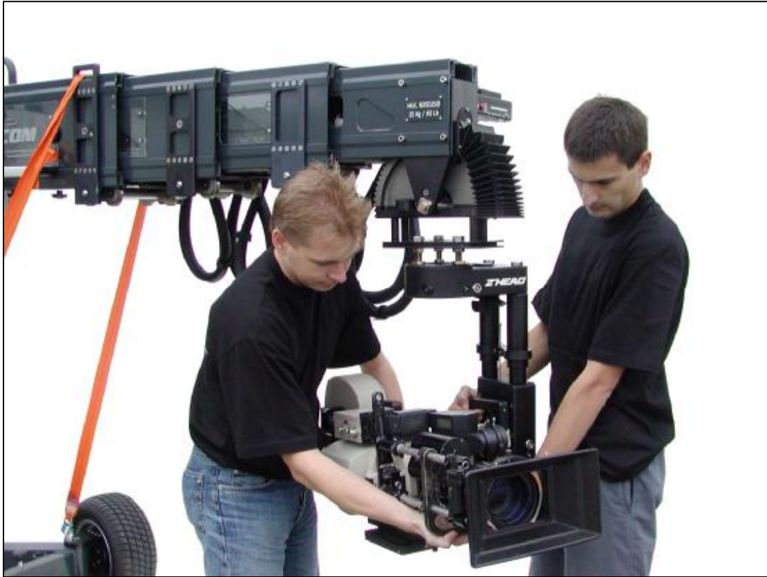
2.9.2.a - Mounting camera at base plate
