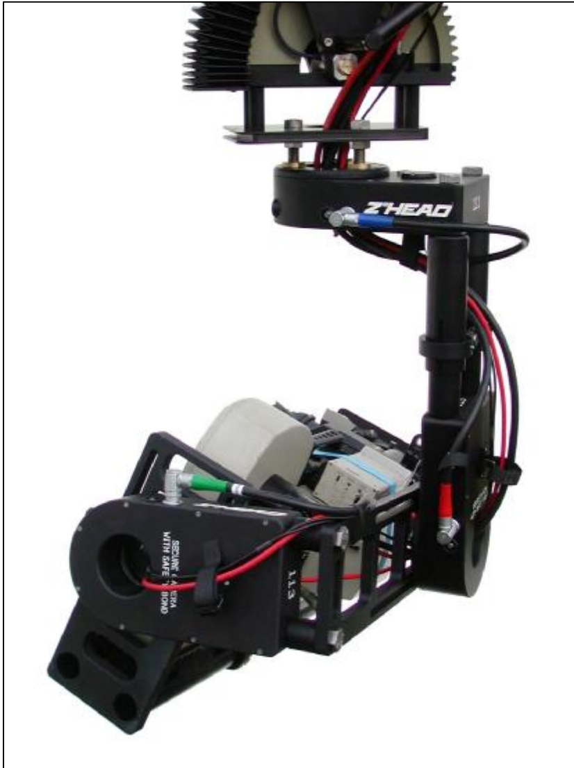
2.9.7.a - Cables at pan, tilt and roll
