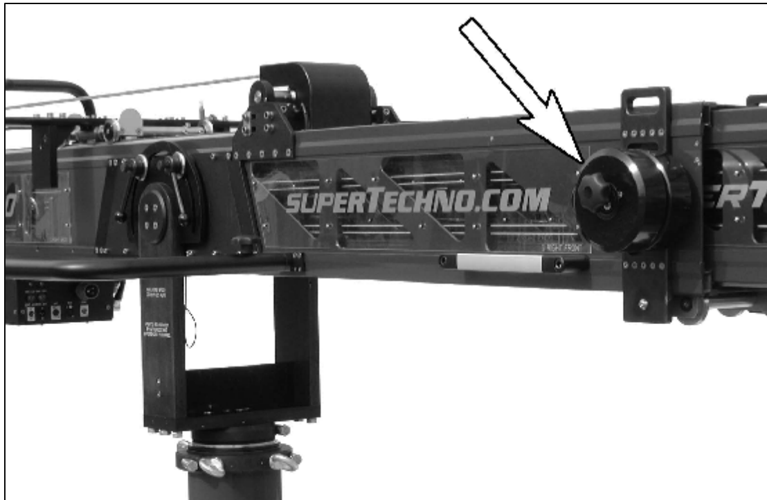
2.7.1.e - Two donuts at first beam front
