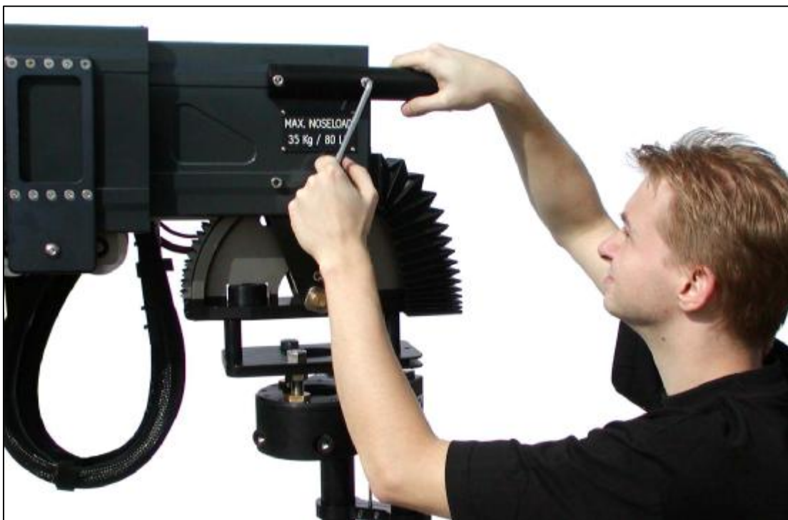
2.15.1.c - Taking off donut holder at autohorizon
