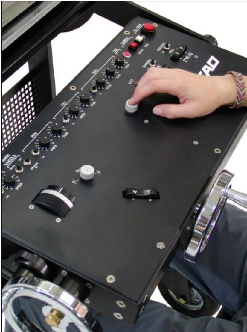
2.16.5.a – Pan-tilt joystick
