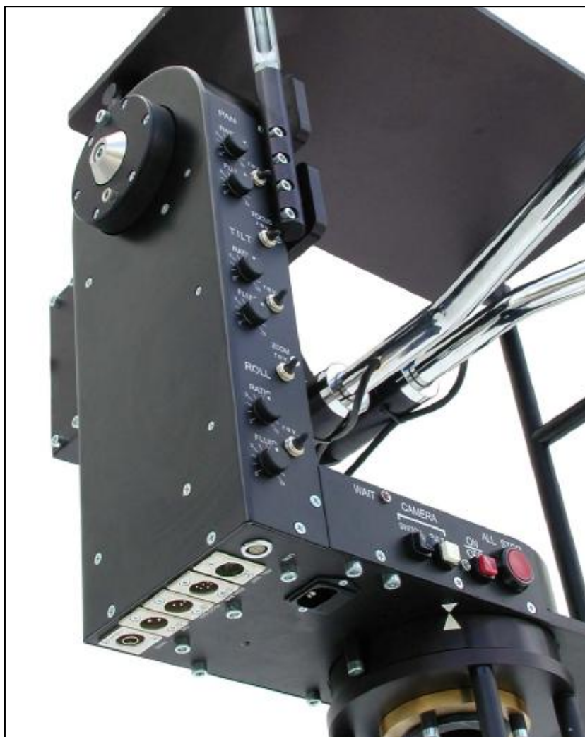
2.18.3. - Connector sockets at pan bars
