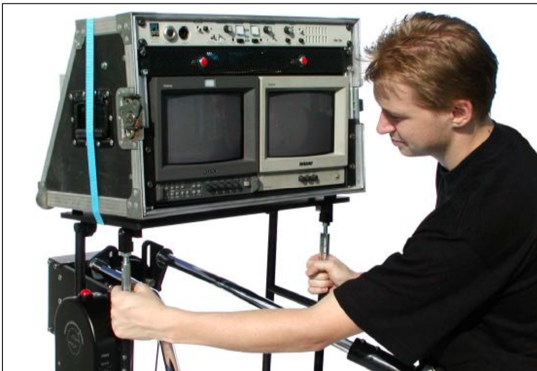
2.18.2.f - Setting the monitor angle with studs
